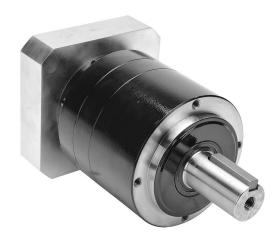
SureGear high-precision planetary gearbox, 15:1 ratio, inline, 32mm diameter output shaft, nominal output torque 120 N-m (1062 lb-in), 2-stage, 120mm frame. For use with SureServo and SureServo2 SV(2)M-210(B) motors.
