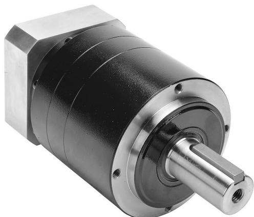
SureGear high-precision planetary gearbox, 15:1 ratio, inline, 32mm diameter output shaft, nominal output torque 120 N-m (1062 lb-in), 2-stage, 120mm frame. For use with SureServo and SureServo2 SV(2)L-210(B) motors.
