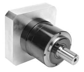
SureGear high-precision planetary gearbox, 10:1 ratio, inline, 32mm diameter output shaft, nominal output torque 120 N-m (1062 lb-in), 1-stage, 120mm frame. For use with SureServo and SureServo2 SV(2)M-220(B) and SV(2)M-230(B) motors.
