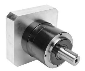
SureGear high-precision planetary gearbox, 5:1 ratio, inline, 32mm diameter output shaft, nominal output torque 180 N-m (1593 lb-in), 1-stage, 120mm frame. For use with SureServo and SureServo2 SV(2)M-220(B) and SV(2)M-230(B) motors.
