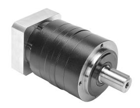
SureGear high-precision planetary gearbox, 15:1 ratio, inline, 22mm diameter output shaft, nominal output torque 50 N-m (443 lb-in), 2-stage, 90mm frame. For use with SureServo and SureServo2 SV(2)L-207(B) motors.
