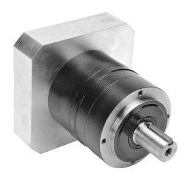
SureGear high-precision planetary gearbox, 10:1 ratio, inline, 22mm diameter output shaft, nominal output torque 50 N-m (443 lb-in), 1-stage, 90mm frame. For use with SureServo and SureServo2 SV(2)M-210(B) motors.
