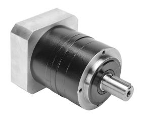
SureGear high-precision planetary gearbox, 10:1 ratio, inline, 22mm diameter output shaft, nominal output torque 50 N-m (443 lb-in), 1-stage, 90mm frame. For use with SureServo and SureServo2 SV(2)L-210(B) motors.
