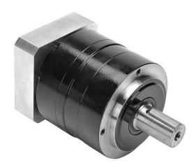
SureGear high-precision planetary gearbox, 10:1 ratio, inline, 22mm diameter output shaft, nominal output torque 50 N-m (443 lb-in), 1-stage, 90mm frame. For use with SureServo and SureServo2 SV(2)L-207(B) motors.
