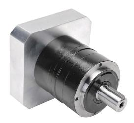
SureGear high-precision planetary gearbox, 5:1 ratio, inline, 22mm diameter output shaft, nominal output torque 75 N-m (664 lb-in), 1-stage, 90mm frame. For use with SureServo and SureServo2 SV(2)M-210(B) motors.
