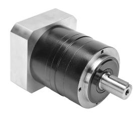
SureGear high-precision planetary gearbox, 5:1 ratio, inline, 22mm diameter output shaft, nominal output torque 75 N-m (664 lb-in), 1-stage, 90mm frame. For use with SureServo and SureServo2 SV(2)L-210(B) motors.
