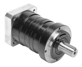
SureGear high-precision planetary gearbox, 25:1 ratio, inline, 16mm diameter output shaft, nominal output torque 27 N-m (239 lb-in), 2-stage, 70mm frame. For use with SureServo and SureServo2 SV(2)L-202(B) and SV(2)L-204(B) motors.
