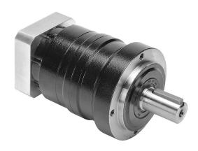
SureGear high-precision planetary gearbox, 15:1 ratio, inline, 16mm diameter output shaft, nominal output torque 18 N-m (159 lb-in), 2-stage, 70mm frame. For use with SureServo and SureServo2 SV(2)L-201(B) motors.
