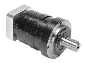
SureGear high-precision planetary gearbox, 15:1 ratio, inline, 16mm diameter output shaft, nominal output torque 18 N-m (159 lb-in), 2-stage, 70mm frame. For use with SureServo and SureServo2 SV(2)L-201(B) motors.
