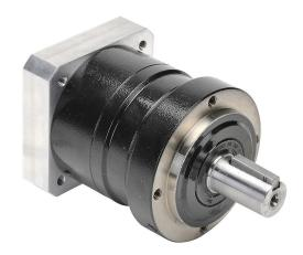
SureGear high-precision planetary gearbox, 10:1 ratio, inline, 16mm diameter output shaft, nominal output torque 18 N-m (159 lb-in), 1-stage, 70mm frame. For use with SureServo and SureServo2 SV(2)L-202(B) and SV(2)L-204(B) motors.
