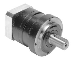
SureGear high-precision planetary gearbox, 10:1 ratio, inline, 16mm diameter output shaft, nominal output torque 18 N-m (159 lb-in), 1-stage, 70mm frame. For use with SureServo and SureServo2 SV(2)L-201(B) motors.
