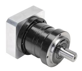
SureGear high-precision planetary gearbox, 5:1 ratio, inline, 16mm diameter output shaft, nominal output torque 27 N-m (239 lb-in), 1-stage, 70mm frame. For use with SureServo and SureServo2 SV(2)L-207(B) motors.
