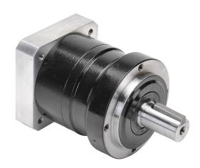
SureGear high-precision planetary gearbox, 5:1 ratio, inline, 16mm diameter output shaft, nominal output torque 27 N-m (239 lb-in), 1-stage, 70mm frame. For use with SureServo and SureServo2 SV(2)L-202(B) and SV(2)L-204(B) motors.
