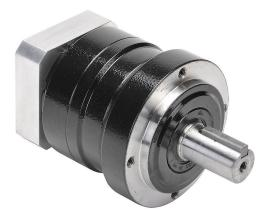
SureGear high-precision planetary gearbox, 5:1 ratio, inline, 16mm diameter output shaft, nominal output torque 27 N-m (239 lb-in), 1-stage, 70mm frame. For use with SureServo and SureServo2 SV(2)L-201(B) motors.
