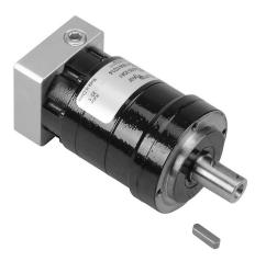
SureGear high-precision planetary gearbox, 25:1 ratio, inline, 12mm diameter output shaft, nominal output torque 9 N-m (80 lb-in), 2-stage, 50mm frame. For use with SureServo and SureServo2 SV(2)L-201(B) motors.
