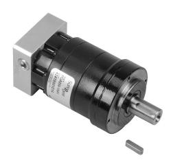
SureGear high-precision planetary gearbox, 15:1 ratio, inline, 12mm diameter output shaft, nominal output torque 6 N-m (53 lb-in), 2-stage, 50mm frame. For use with SureServo and SureServo2 SV(2)L-201(B) motors.
