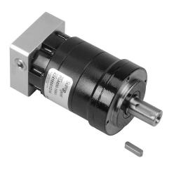
SureGear high-precision planetary gearbox, 15:1 ratio, inline, 12mm diameter output shaft, nominal output torque 6 N-m (53 lb-in), 2-stage, 50mm frame. For use with SureServo and SureServo2 SV(2)L-201(B) motors.
