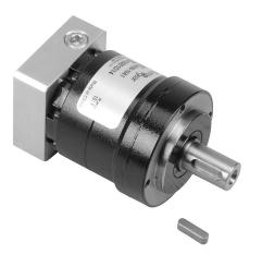
SureGear high-precision planetary gearbox, 10:1 ratio, inline, 12mm diameter output shaft, nominal output torque 6 N-m (53 lb-in), 1-stage, 50mm frame. For use with SureServo and SureServo2 SV(2)L-201(B) motors.
