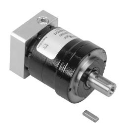
SureGear high-precision planetary gearbox, 5:1 ratio, inline, 12mm diameter output shaft, nominal output torque 9 N-m (80 lb-in), 1-stage, 50mm frame. For use with SureServo and SureServo2 SV(2)L-201(B) motors.
