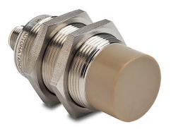
AutomationDirect inductive proximity sensor, tubular, 30mm diameter x 70mm body, 316L stainless steel housing, PNP, N.O. output, 22mm sensing distance, non-flush, 100 Hz switching frequency, IP68 IP69K, 4-pin M12 quick-disconnect.
