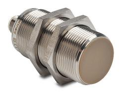
AutomationDirect inductive proximity sensor, tubular, 30mm diameter x 70mm body, 316L stainless steel housing, PNP, N.O. output, 15mm sensing distance, flush, 50 Hz switching frequency, IP68 IP69K, 4-pin M12 quick-disconnect.
