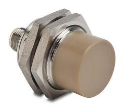
AutomationDirect inductive proximity sensor, tubular, 30mm diameter x 50mm body, 316L stainless steel housing, PNP, N.O. output, 22mm sensing distance, non-flush, 100 Hz switching frequency, IP68 IP69K, 4-pin M12 quick-disconnect.
