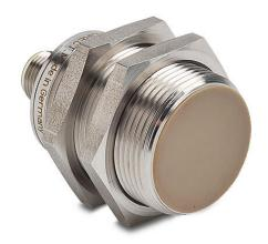
AutomationDirect inductive proximity sensor, tubular, 30mm diameter x 50mm body, 316L stainless steel housing, PNP, N.O. output, 14mm sensing distance, flush, 50 Hz switching frequency, IP68 IP69K, 4-pin M12 quick-disconnect.
