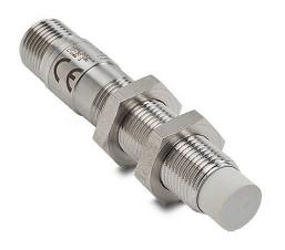
Micro Detectors inductive proximity sensor, tubular, 12mm diameter x 64.8mm body, 316L stainless steel housing, PNP, N.O./ N.C. complementary outputs, 8mm sensing distance, non-flush, 2 kHz switching frequency, IP67 IP68 IP69K, 4-pin M12 quickdisconnect.
