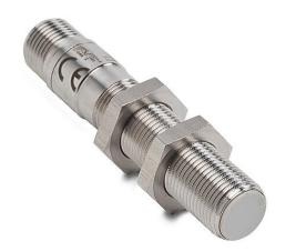
Micro Detectors inductive proximity sensor, tubular, 12mm diameter x 64.8mm body, 316L stainless steel housing, PNP, N.O./ N.C. complementary outputs, 4mm sensing distance, flush, 2 kHz switching frequency, IP67 IP68 IP69K, 4-pin M12 quick-disconnect.
