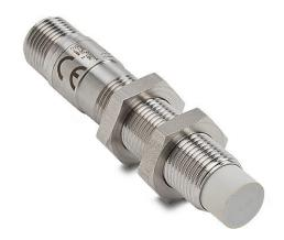
Micro Detectors inductive proximity sensor, tubular, 12mm diameter x 64.8mm body, 316L stainless steel housing, PNP, N.O./ N.C. complementary outputs, 4mm sensing distance, non-flush, 2 kHz switching frequency, IP67 IP68 IP69K, 4-pin M12 quick-disconnect.
