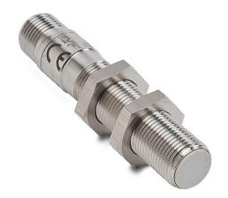
Micro Detectors inductive proximity sensor, tubular, 12mm diameter x 64.8mm body, 316L stainless steel housing, PNP, N.O./ N.C. complementary outputs, 2mm sensing distance, flush, 2 kHz switching frequency, IP67 IP68 IP69K, 4-pin M12 quick-disconnect.
