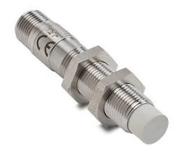
Micro Detectors inductive proximity sensor, tubular, 12mm diameter x 64.8mm body, 316L stainless steel housing, NPN, N.O./ N.C. complementary outputs, 8mm sensing distance, non-flush, 2 kHz switching frequency, IP67 IP68 IP69K, 4-pin M12 quick-disconnect.
