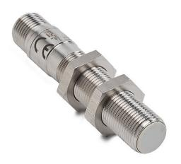
Micro Detectors inductive proximity sensor, tubular, 12mm diameter x 64.8mm body, 316L stainless steel housing, NPN, N.O./ N.C. complementary outputs, 4mm sensing distance, flush, 2 kHz switching frequency, IP67 IP68 IP69K, 4-pin M12 quick-disconnect.
