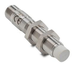
Micro Detectors inductive proximity sensor, tubular, 12mm diameter x 64.8mm body, 316L stainless steel housing, NPN, N.O./ N.C. complementary outputs, 4mm sensing distance, non-flush, 2 kHz switching frequency, IP67 IP68 IP69K, 4-pin M12 quickdisconnect.
