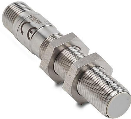
Micro Detectors inductive proximity sensor, tubular, 12mm diameter x 64.8mm body, 316L stainless steel housing, NPN, N.O./N.C. complementary outputs, 2mm sensing distance, flush, 2 kHz switching frequency, IP67 IP68 IP69K, 4-pin M12 quick-disconnect.
