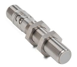
Micro Detectors inductive proximity sensor, tubular, 12mm diameter x 64.8mm body, 316L stainless steel housing, NPN, N.O./ N.C. complementary outputs, 2mm sensing distance, flush, 2 kHz switching frequency, IP67 IP68 IP69K, 4-pin M12 quick-disconnect.
