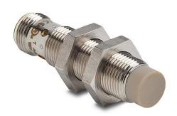
AutomationDirect inductive proximity sensor, tubular, 12mm diameter x 45mm body, 316L stainless steel housing, PNP, N.O. output, 7mm sensing distance, non-flush, 800 Hz switching frequency, IP68 IP69K, 4-pin M12 quick-disconnect.
