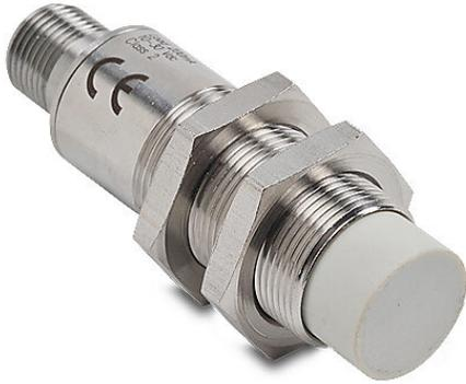
Micro Detectors inductive proximity sensor, tubular, 18mm diameter x 63mm body, 316L stainless steel housing, PNP, N.O./N.C. complementary outputs, 12mm sensing distance, non-flush, 1.5 kHz switching frequency, IP67 IP68 IP69K, 4-pin M12 quick-disconnect.
