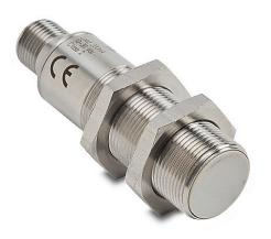
Micro Detectors inductive proximity sensor, tubular, 18mm diameter x 63mm body, 316L stainless steel housing, PNP, N.O./ N.C. complementary outputs, 8mm sensing distance, flush, 1.5 kHz switching frequency, IP67 IP68 IP69K, 4-pin M12 quickdisconnect.
