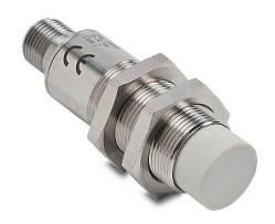
Micro Detectors inductive proximity sensor, tubular, 18mm diameter x 63mm body, 316L stainless steel housing, PNP, N.O./ N.C. complementary outputs, 8mm sensing distance, non-flush, 1.5 kHz switching frequency, IP67 IP68 IP69K, 4-pin M12 quick-disconnect.
