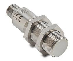
Micro Detectors inductive proximity sensor, tubular, 18mm diameter x 63mm body, 316L stainless steel housing, PNP, N.O./ N.C. complementary outputs, 5mm sensing distance, flush, 1.5 kHz switching frequency, IP67 IP68 IP69K, 4-pin M12 quick-disconnect.
