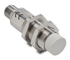
Micro Detectors inductive proximity sensor, tubular, 18mm diameter x 63mm body, 316L stainless steel housing, NPN, N.O./ N.C. complementary outputs, 12mm sensing distance, non-flush, 1.5 kHz switching frequency, IP67 IP68 IP69K, 4-pin M12 quickdisconnect.
