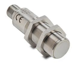
Micro Detectors inductive proximity sensor, tubular, 18mm diameter x 63mm body, 316L stainless steel housing, NPN, N.O./ N.C. complementary outputs, 8mm sensing distance, flush, 1.5 kHz switching frequency, IP67 IP68 IP69K, 4-pin M12 quick-disconnect.
