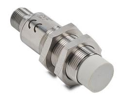
Micro Detectors inductive proximity sensor, tubular, 18mm diameter x 63mm body, 316L stainless steel housing, NPN, N.O./ N.C. complementary outputs, 8mm sensing distance, non-flush, 1.5 kHz switching frequency, IP67 IP68 IP69K, 4-pin M12 quick-disconnect.
