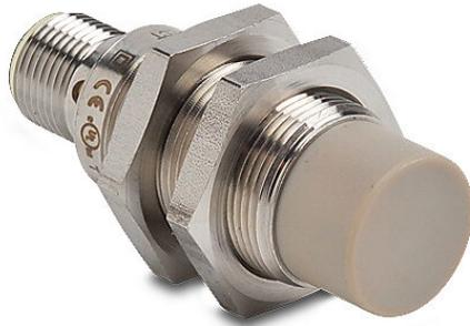
AutomationDirect inductive proximity sensor, tubular, 18mm diameter x 51mm body, 316L stainless steel housing, PNP, N.O. output, 12mm sensing distance, non-flush, 300 Hz switching frequency, IP68 IP69K, 4-pin M12 quick-disconnect.
