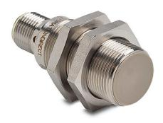
AutomationDirect inductive proximity sensor, tubular, 18mm diameter x 46mm body, 316L stainless steel housing, PNP, N.O. output, 8mm sensing distance, flush, 600 Hz switching frequency, IP68 IP69K, 4-pin M12 quick-disconnect.
