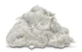
Killark packing fiber, 1-pound container. For use with hazardous location sealing fittings.
