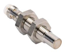
ProSense inductive proximity sensor, tubular, 8mm diameter x 45mm body, stainless steel housing, PNP, N.O. output, 5mm sensing distance, non-flush, 500 Hz switching frequency, IP65 IP66 IP67 IP68 IP69K, 3-pin M8 quick-disconnect.
