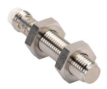
ProSense inductive proximity sensor, tubular, 8mm diameter x 45mm body, stainless steel housing, PNP, N.O. output, 3mm sensing distance, semi-flush, 250 Hz switching frequency, IP65 IP66 IP67 IP68 IP69K, 3-pin M8 quick-disconnect.
