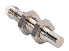
ProSense inductive proximity sensor, tubular, 8mm diameter x 45mm body, stainless steel housing, NPN, N.O. output, 5mm sensing distance, non-flush, 500 Hz switching frequency, IP65 IP66 IP67 IP68 IP69K, 3-pin M8 quick-disconnect.
