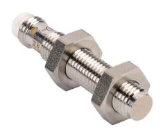
ProSense inductive proximity sensor, tubular, 8mm diameter x 45mm body, stainless steel housing, NPN, N.O. output, 3mm sensing distance, semi-flush, 250 Hz switching frequency, IP65 IP66 IP67 IP68 IP69K, 3-pin M8 quick-disconnect.
