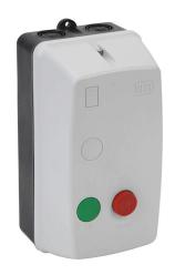
WEG Electric PESWS series manual motor starter, pushbutton, 9A, 2-pole, 120 VAC (50/60Hz) coil voltage, thermal overload, 5.6-8.0A Adjustable, NEMA 4/4X.
