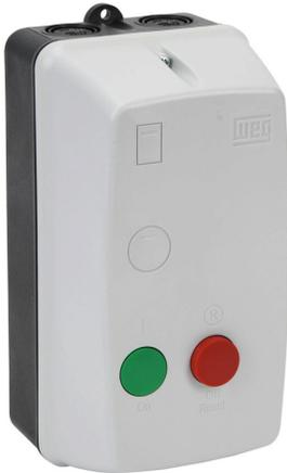
WEG Electric PESWS series manual motor starter, pushbutton, 9A, 2-pole, 120 VAC (50/60Hz) coil voltage, thermal overload, 2.8-4.0A Adjustable, NEMA 4/4X.
